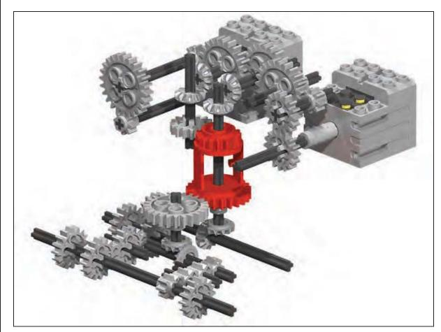
Drive gear arrangements for both tracks on the older JS70 model – the motors are located at the rear of the superstructure. A differential case, shown in red, goes through the center of the turntable (not shown) and acts as the outer shaft for the concentric drive system, eventually leading to the drive sprocket for the left track. The axle going through the center of the red differential case can be driven independently of it and drives the sprocket for the right track.
