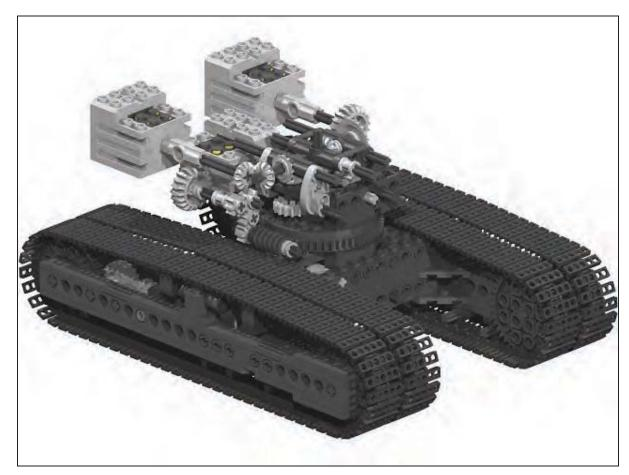
All three motors, one driving each track and another for slewing, are located in the rear of the superstructure. In additional to allowing infinite slew, this also makes them function as effective counterweights, rather than dead weight in the undercarriage.
